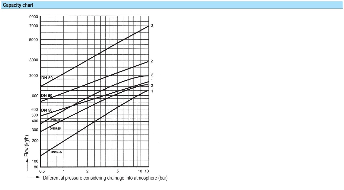
The capacity chart shows the maximum capacity at factory setting.
