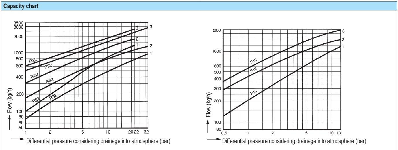
The capacity chart shows the maximum capacity at factory setting. (Other factory-settings for the sub-cooling on request.)
