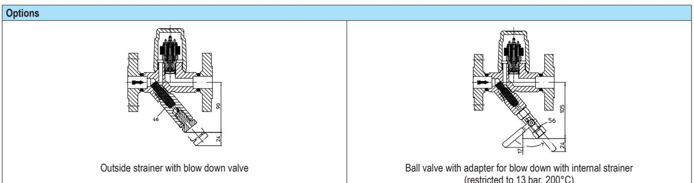
**Bimetallic steam trap (Forged steel, High temperature steel, Stainless steel)**
