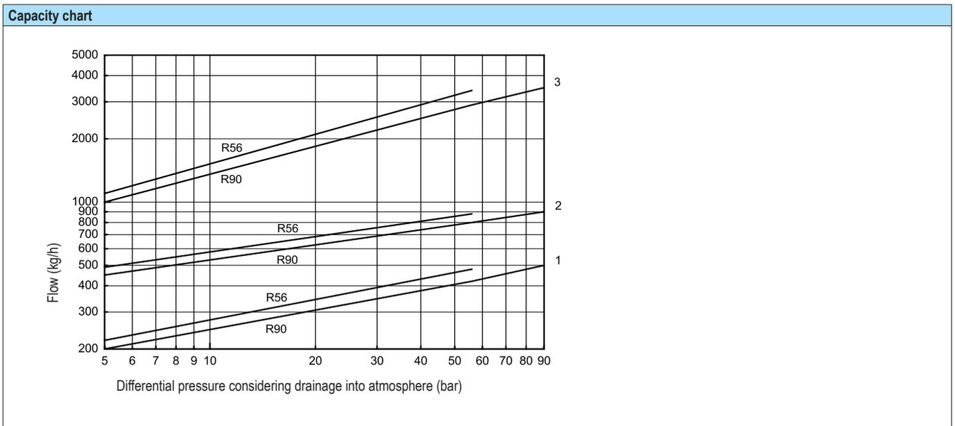
The capacity chart shows the maximum flow at factory setting.
