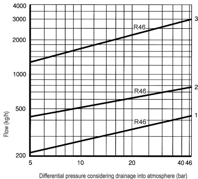
The capacity chart shows the maximum capacity at factory setting.
