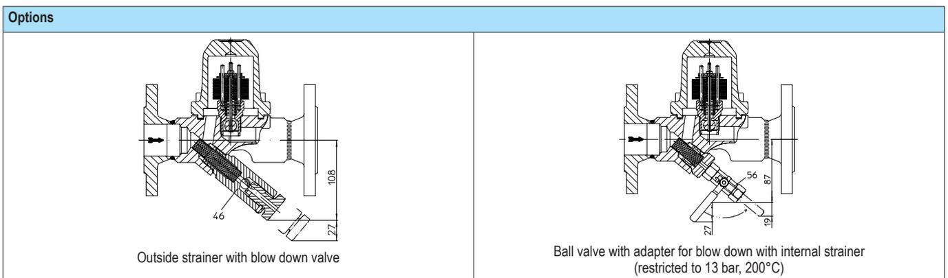
**Bimetallic steam trap (High temperature steel)**
