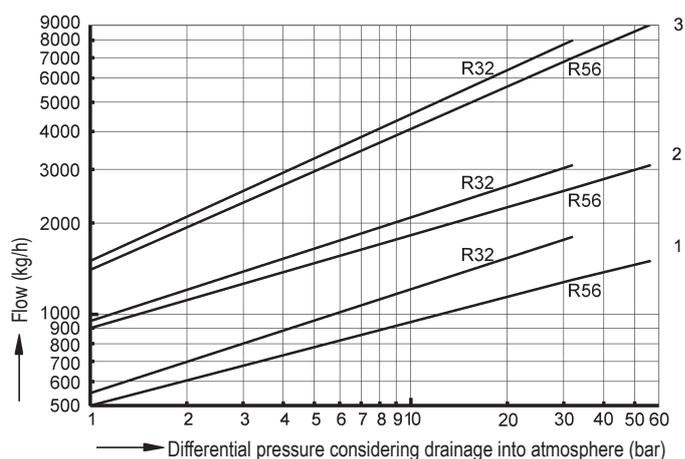
The capacity chart shows the maximum flow at factory setting.
