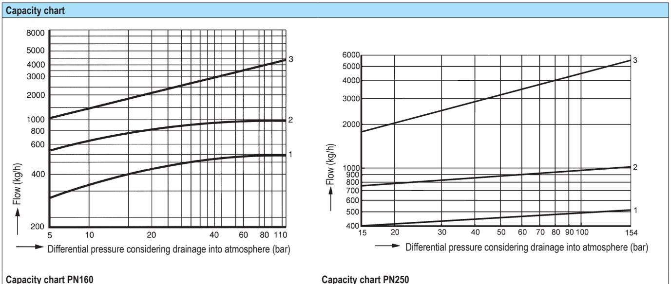
The capacity chart shows the maximum capacity at factory setting.
